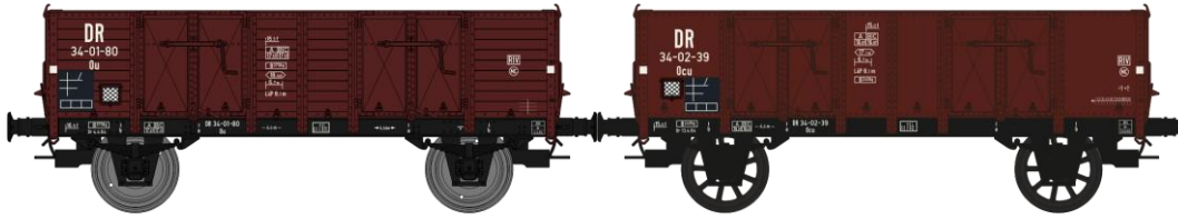
Réf. WB-275 - Set of 2 Wagons OPEN CAR Era.IV DR W-010-K-02 Wood, Cushion wheelboxess, Plain wheels, N° 34-01-80 Ou W-010-O-04 Steel plate, Cushion wheelboxess, Spoked wheels, N° 34-02-39 Ocu
