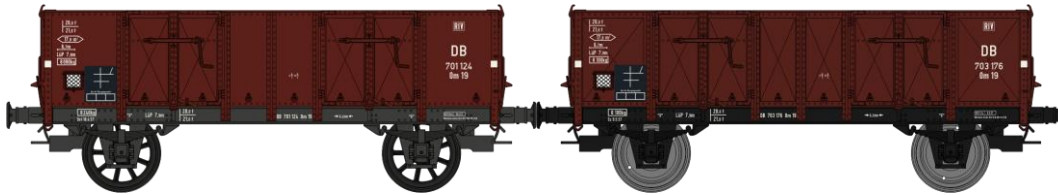
Réf. WB-270 - Set of 2 Wagons OPEN CAR Era.III DB W-010-O-02 Steel plate, Cushion wheelboxess, Spoked wheels, N° 701 124 Om19 W-010-J-01 Steel buckled plate, Cushion wheelboxess, Plain wheels, N° 703 176 Om19
